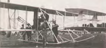
The Wrights mastered aircraft control with their gliders (1902 model above) then added propulsion. Below—1909 Military Wright Flyer. Ribbon on front spar served as drift indicator.
