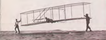
The Wrights mastered aircraft control with their gliders (1902 model above) then added propulsion. Below—1909 Military Wright Flyer. Ribbon on front spar served as drift indicator.
