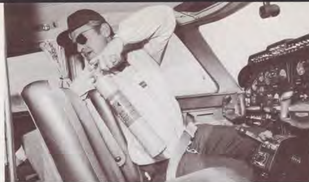
Plain water in a pressurized container remains the most effective fire fighting agent for cabin fires. It is fast acting, non-toxic, non-corrosive and leaves no residue.
