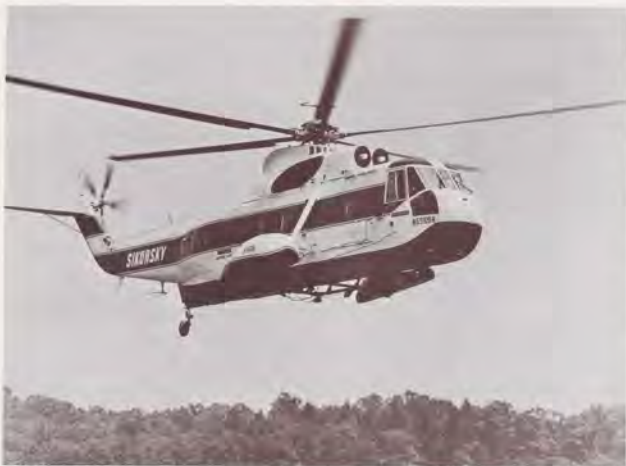
Amphibious Sikorsky S-61N is typical of multi-engine helicopters now active in air carrier service. S-61N can carry crew of two and 28 passengers at 140 mph over 248 miles.
