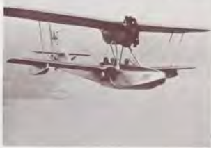
Above—stainless steel Pioneer skims across Long Island Sound on its maiden flight, Oct. 4, 1931. Bottom left—John C. Whitesell, project engineer for first successful steel plane, is center man in trio aboard two-place aircraft. Bottom right—at 1,500 pounds, the stainless steel airplane was lighter than the all-wood Savoia Marchetti SM-56 model. Budd engineers used revolutionary shot weld process to join thousands of components into light, strong airframe. Examined during renovation 37 years later, integrity of welds was intact although carbon steel bolts used to join wings and engine mounts were rusted away.
