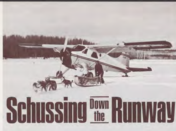
Versatility of ski/wheel equipped aircraft is taking business away from the dogs in northern Canada and Alaska. Below —wheel replacement skis are used extensively by bush pilots for sport and business flying.
