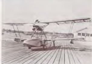
Above—stainless steel Pioneer skims across Long Island Sound on its maiden flight, Oct. 4, 1931. Bottom left—John C. Whitesell, project engineer for first successful steel plane, is center man in trio aboard two-place aircraft. Bottom right—at 1,500 pounds, the stainless steel airplane was lighter than the all-wood Savoia Marchetti SM-56 model. Budd engineers used revolutionary shot weld process to join thousands of components into light, strong airframe. Examined during renovation 37 years later, integrity of welds was intact although carbon steel bolts used to join wings and engine mounts were rusted away.
