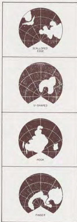
Characteristic radar returns showing severe storm activity. From top: scalloped edge image depicts hail; a U-shaped pattern is related to tornadoes; a prominent hook is associated with high turbulence and a finger return is linked to violent storm activity.
