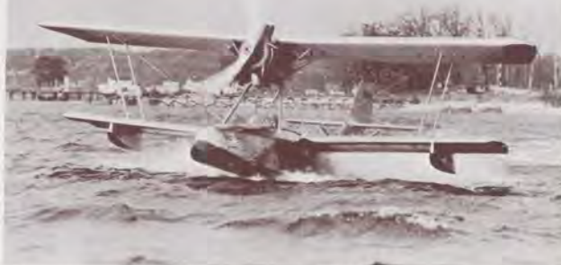
Above—stainless steel Pioneer skims across Long Island Sound on its maiden flight, Oct. 4, 1931. Bottom left—John C. Whitesell, project engineer for first successful steel plane, is center man in trio aboard two-place aircraft. Bottom right—at 1,500 pounds, the stainless steel airplane was lighter than the all-wood Savoia Marchetti SM-56 model. Budd engineers used revolutionary shot weld process to join thousands of components into light, strong airframe. Examined during renovation 37 years later, integrity of welds was intact although carbon steel bolts used to join wings and engine mounts were rusted away.
