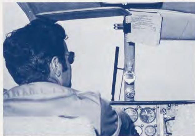
Emergency checklist clipped on backside of a sun visor or other handy storage place may be a lifesaver when fast reaction is needed. Print should be large, instructions concise.
