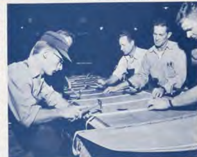
Applying plywood skin is a team effort. Surface will later be covered with dacron. Below—plywood leading edge is held firmly in place on the ribs by straps on the jig.
