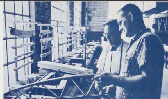
Strength of all-wood rib compares favorably with metal construction. Below—all-wood wing combines strength with light weight and ease of construction.
