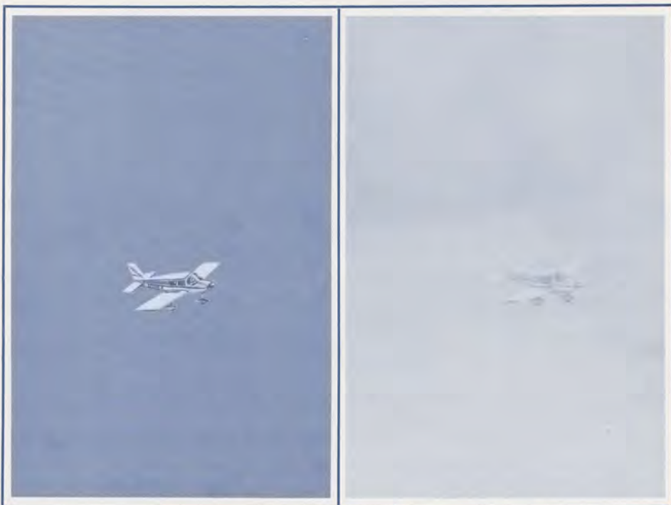
An aircraft seen against a hazy background loses its sharp outlines and may appear deceptively distant to the viewer.
