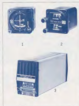
One simple area navigation system uses (1) course indicator, (2) VORTAC offset controller, and (3) a computer.
