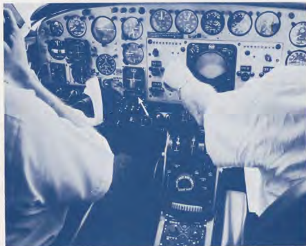
Pilot uses airborne computer to dial selected way point as he would set OMNI heading to VOR checkpoint on airway. Arrow indicates track and distance display.
