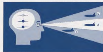
Aircraft "B" (out of focus), registers as distant as "A", although it is much closer. Aircraft "C" (in periphery) seems smaller and less distinct even though it is as close as "A".
