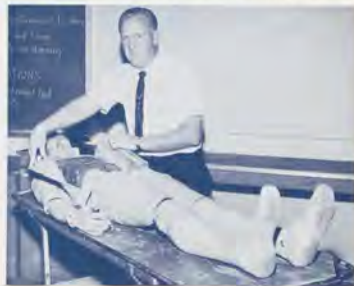
Above—FAA survival expert E. B. McFadden with anthropomorphic dummy used in immersion tests. Antenna on skull transmits telemetered data from transmitter in chest to boat or shore-based monitors. Below—McFadden shows radio in dummy's "chest."
