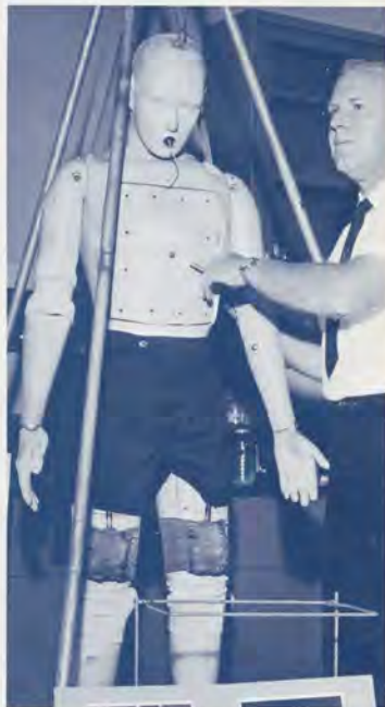
Above—FAA survival expert E. B. McFadden with anthropomorphic dummy used in immersion tests. Antenna on skull transmits telemetered data from transmitter in chest to boat or shore-based monitors. Below—McFadden shows radio in dummy's "chest."
