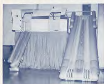
Above—experimental plastic smoke hood can withstand temperatures up to 1,472°F before charring. Below—latest model inflatable escape chute (r), designed for Boeing 747, has safety patches on the bottom to slow passenger slide and prevent injury.
