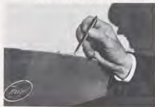
Extend prop life by having a mechanic file sharp nicks into shallow depressions.
