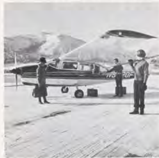
Careless storage of skis and other gear can alter plane's center of gravity.
