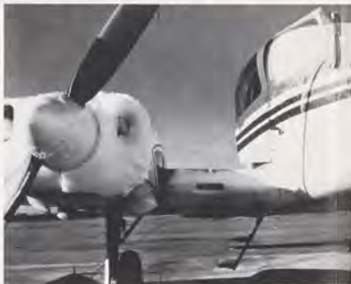
Engine cowl and windshield covers can prevent ice buildup, cut preflight time.
