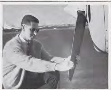
Prop preflight includes twisting and bending blades to detect looseness. Check for nicks, cuts, bruises and security of prop spinner mounting.
