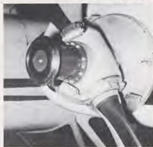
Below, left. Whenever spinner is removed, inspect safeties, signs of excessive oil leakage. Right. In many cases, severely bent props can be repaired but all work must be done by qualified mechanics in accordance with FAA standards.
