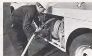
Hose should be checked for wear.
