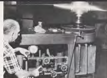
Left—General aviation props include fixed pitch wood and aluminum (left, on table) and ground adjustable steel props. Full feathering hydromatic prop hangs from sling. Above—Prop is tested for oil leaks after assembly.
