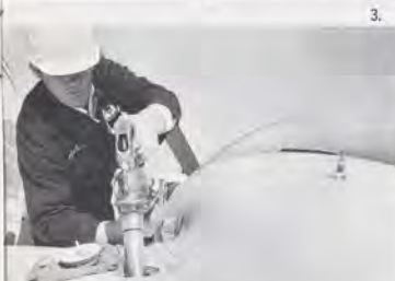
1. First step (above) is attaching cable from truck to ground post. 2. Second cable goes to aircraft to wheel or strut. 3. Third cable from home nozzle is snapped on wing clip.
