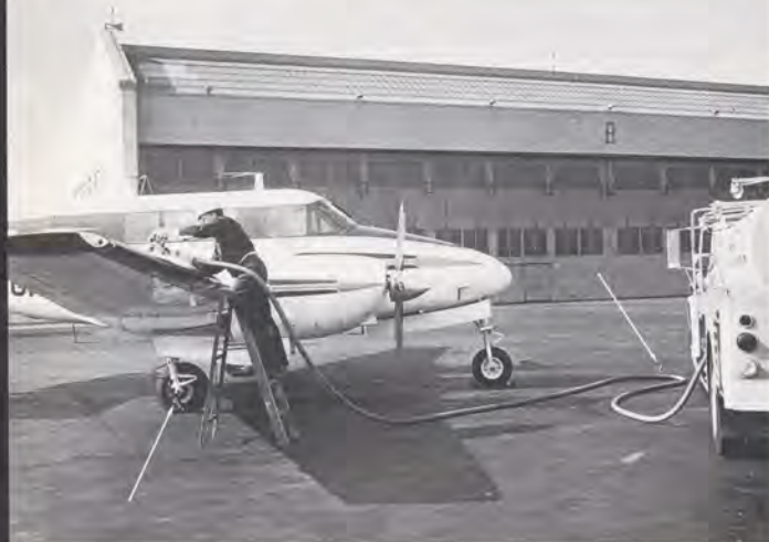
Truck is grounded to sunken post, airplane is bonded to truck, wing is bonded to nozzle.
