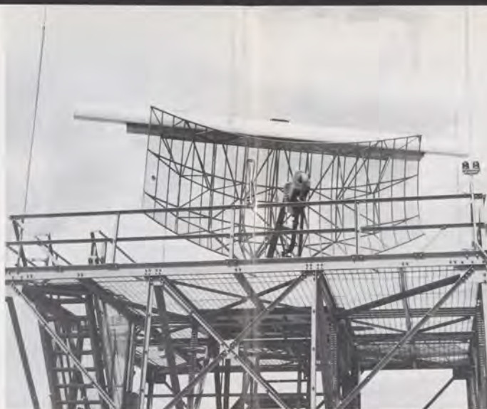
Above—The parabolic antenna transmits and receives primary radar. The horizontal bar mounted above is the interrogator for radar beacon. Below—Air Traffic controllers monitoring the course of aircraft on instrument flight plans. Flight data strips in rack are sequenced according to the latest flight information transmitted by teletype or radio.
