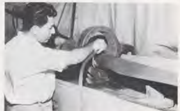
Above—Magnafluxing for hidden cracks is standard practice in prop overhaul. Right—"Dead" props often come to life.
