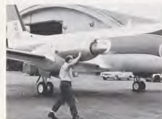
Top—the business end of a business jet can be just as dangerous as an airline engine. Bottom—beware the prop, and don't forget the ear muffs when working around turbo-prop engines.
