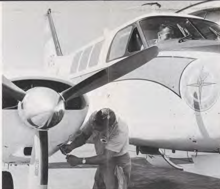
Above—a potentially dangerous situation. Mechanics working on an engine should make certain no one enters the cockpit or handles controls without his knowledge. An accidentally flipped switch could spin the prop.
