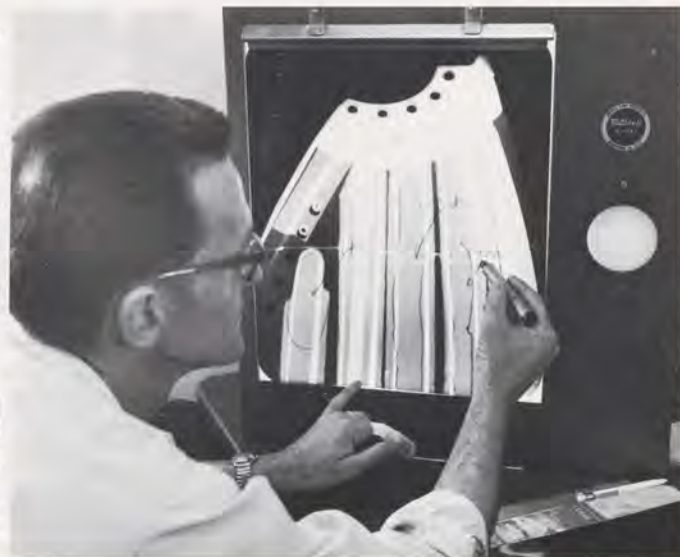
Above, Fluorescent dye penetrant kit can be easily carried to work site. Right, Cracks in clam shell thrust reversers show up clearly under X-ray examination.
