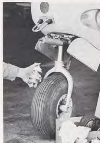
Above, Fluorescent dye penetrant kit can be easily carried to work site. Right, Cracks in clam shell thrust reversers show up clearly under X-ray examination.
