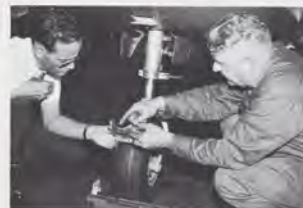
This failed nosewheel stop will be reported in AIDS to warn mechanics.
