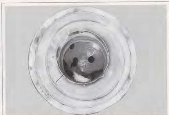
Above. Broken muffler baffle plate restricts engine power. Below. Crack, concealed by heater shroud need not be large to admit dangerous CO to cabin.
