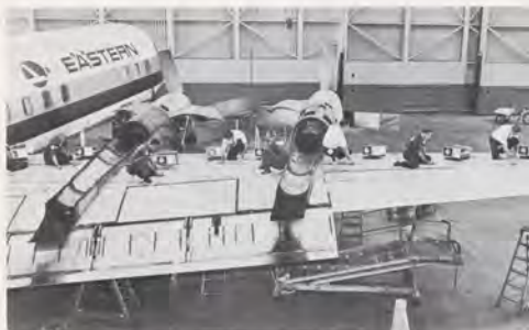
Eight inspectors swarm over Electra turboprop wing with ultrasonic "black boxes" searching for internal structural flaws.
