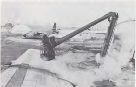
Above: Preheating the engine and cabin is a prime safety precaution that makes for easier engine starting and more comfortable flight. Below: Air Force mechanics apply de-icing fluid from safe vantage point on "cherry picker" lift.
