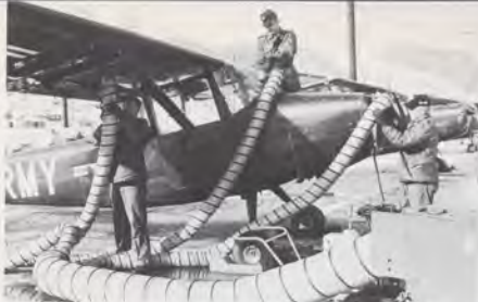
Above: Preheating the engine and cabin is a prime safety precaution that makes for easier engine starting and more comfortable flight. Below: Air Force mechanics apply de-icing fluid from safe vantage point on "cherry picker" lift.
