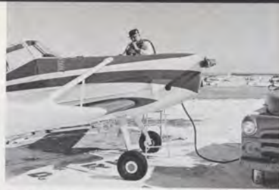
Above: Before hangaring plane after winter flight, top the fuel tanks to prevent condensation. Below: When plane remains idle between flights, condensation can quickly accumulate dangerous amounts of water. Drain your sumps.
