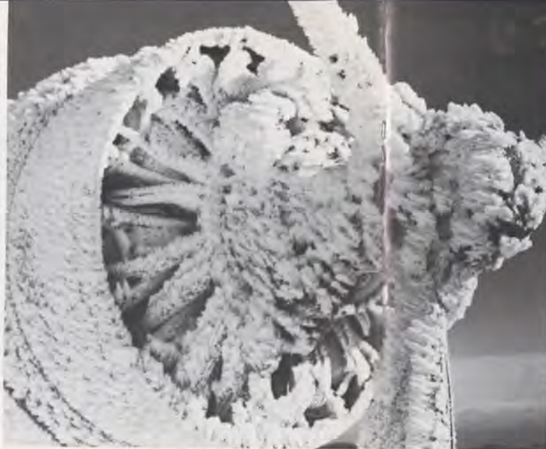
An "ice vise" accumulated on this engine after brief exposure during sleet storm.
