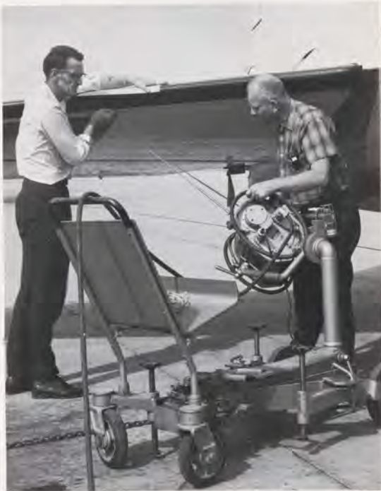
Portable X-ray, mobile as a tool box, being sited for DC-3 stabilizer check.
