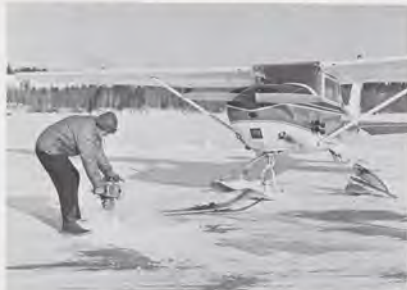
Above: Before hangaring plane after winter flight, top the fuel tanks to prevent condensation. Below: When plane remains idle between flights, condensation can quickly accumulate dangerous amounts of water. Drain your sumps.
