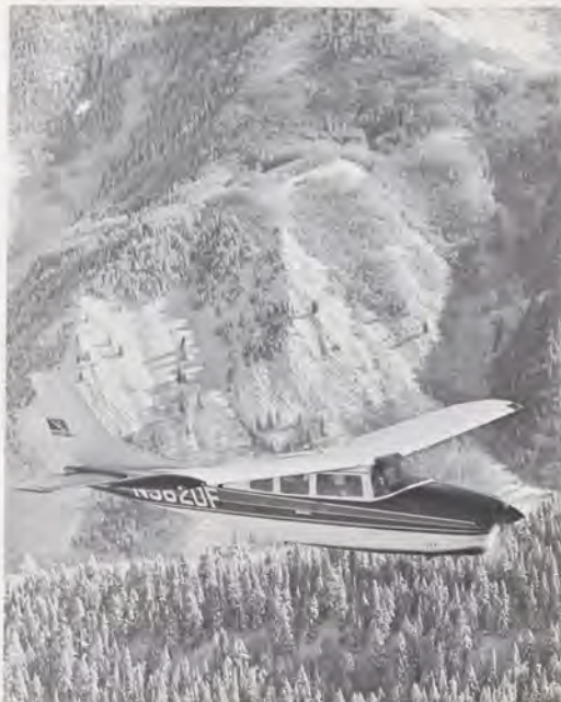
Left: A single-engine aircraft soars easily over the Continental Divide in winter, when cold, dense air gives improved aircraft performance. Above: In the heat of summer, aircraft struggle harder to stay airborne. Once above ground effects, climb rate for non-supercharged Bonanza is cut severely by high density altitude.
