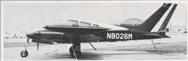
Identification number must be at least 12 inches high, painted on both sides of fuselage or rudder.
