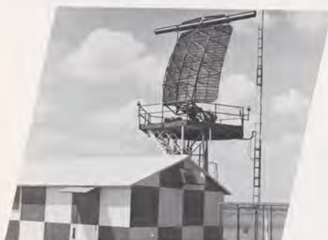
Airport Surveillance Radar "sees" you up to 40 miles.
