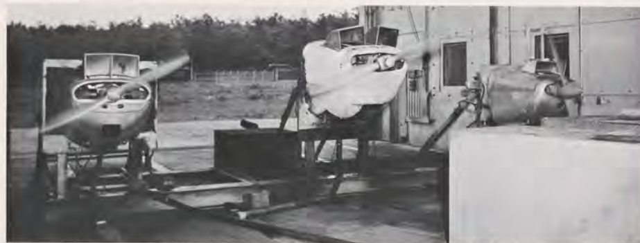
These engines at NAFEC, operating at takeoff, high cruise and idling powers, are prime research tools in studies of exhaust systems and CO.
