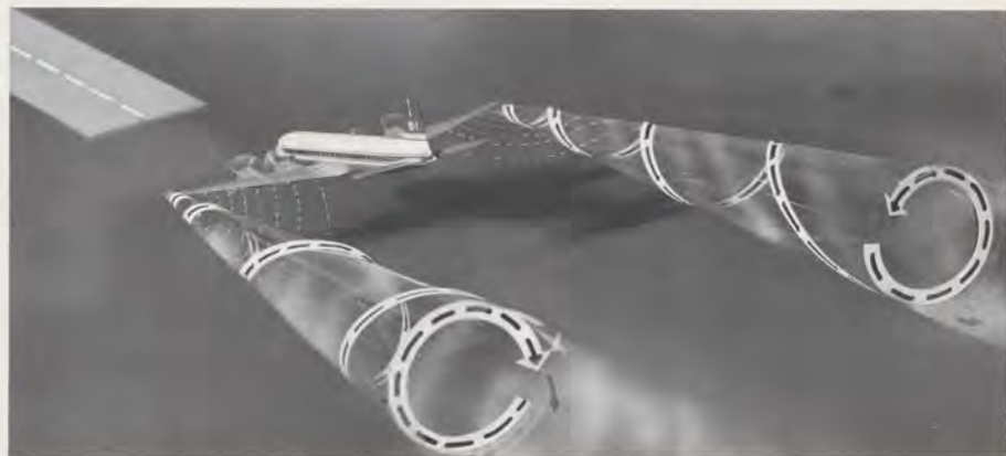
Dotted spiral arrows emanating from wing tips indicate the counter rotation of vortices—invisible downward whirlpools of air—trailing behind plane.
