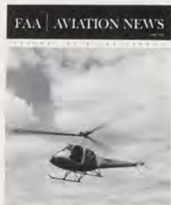
The new Enstrom F28, a three-place 100-mile-an-hour helicopter, was recently issued a type certificate by the Federal Aviation Agency. The F28 was conceived, designed and built in four and a half years.
