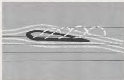
As air spills over the wing, above and below, distinct vortices are formed and trail behind each wing tip. The severity of the turbulence is related to the size, weight, wing span and speed of the aircraft.
