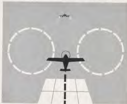
These diagrams indicate how foolish it would be for the pilot of a light plane to try to penetrate vortices behind a heavily loaded aircraft inasmuch as the forces could exceed his plane's climb or control capability. Also, the strain could cause structural failure.
