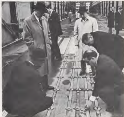
the test lights by sliding along grooves, simulating approach and landing. Above right, engineers check runway lights which, like the 1,000-foot runway, have been scaled to one-tenth size giving the impression of a 10,000-foot runway. The fog used in experiments is produced by piping compressed air and steam into the tunnel-like chamber.
