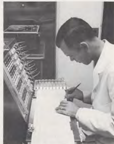
Reading clockwise, from upper left: ● A CARI doctor attaches 12 electrical leads to the panel behind the subject's head. The leads transmit electrical impulses to the EEG machine which records six areas of the brain, plus eye movements. ● Mockup cockpit is shrouded to simulate the effect of a rotating beacon when an aircraft penetrates a cloud formation. ● Technician indicates the normal stylus trace of the horizontal eye movement before beginning test. ● A CARI employee is wired for a "flight" in the mockup by an electroencephalograph technician.
