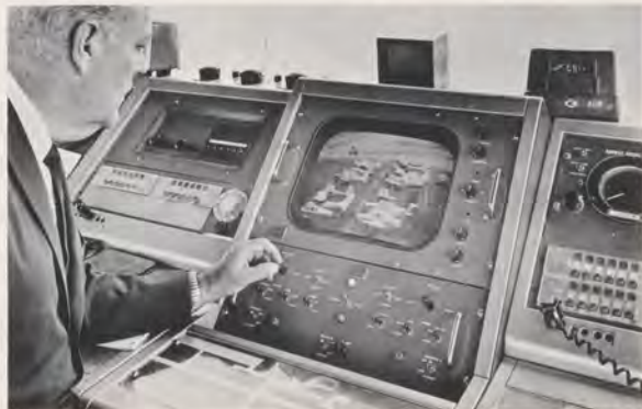
FAA Systems Research and Development Service personnel conducted a series of tests of closed circuit television blind-spot surveillance at Salt Lake City's Municipal Airport No. 1. The remote-control TV cameras were located at heights of 45 and 65 feet to scan areas where visibility from the tower is restricted.
