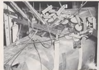
Above: Simulated flight loads are applied simultaneously to the fuselage and wing panel. Right: A "whiffle tree" is used to distribute pressure. Bottom: Landing gear drop tests check the response of the shock absorber.
