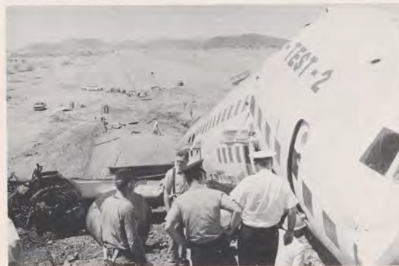
Fractured and battered, but still intact, the fuselage of the aircraft came to rest on the second hill.
