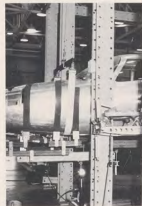
Above: Simulated flight loads are applied simultaneously to the fuselage and wing panel. Right: A "whiffle tree" is used to distribute pressure. Bottom: Landing gear drop tests check the response of the shock absorber.
