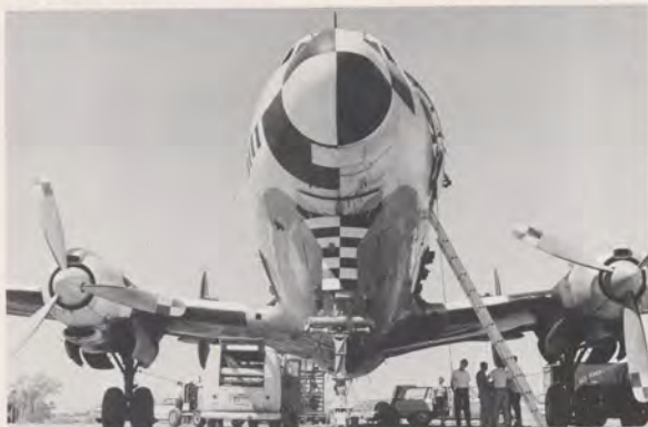
Above—Super Constellation is poised on the guide rail while engineers make final preparations aboard the plane. Below—The Connie throws up a cloud of dust as it is deliberately crashed into man-made barriers simulating a crash landing accident at the Deer Valley Airport test site.
