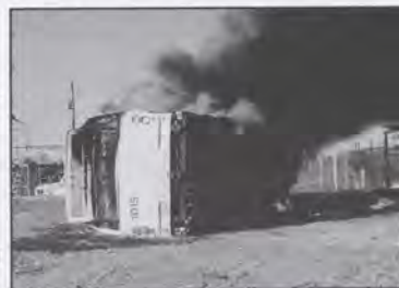
After the Fire-Life Safety Seminar, the Atlanta MARTA bus was set ablaze to compare burn time with evacuation time.
