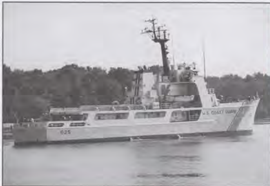
The newly recommissioned Coast Guard Cutter Venturous has an overall length of 210'6", a beam of 34', a draft of 10'8", and displaces 1050 tons. The Cutter is powered by two 2500 horsepower American locomotive marine-gear diesel engines and is capable of 18 knot sustained speed in moderate seas. Twin controllable pitch propellers and rudders give Venturous a high degree of maneuverability. Venturous carries an all volunteer crew composed of 12 officers, six chief petty officers and 64 enlisted personnel. (Official USCG photo by SN J. Travis Parks, Coast Guard YARD.)
