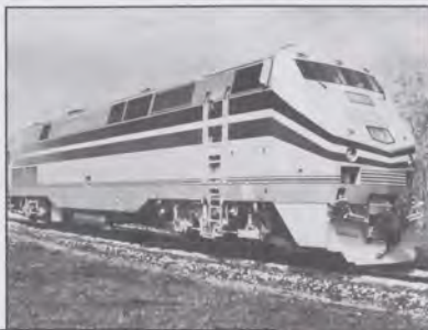
Above: Brunel Winner for Locomotive Design. Amtrak's AMD-103 Genesis Locomotive Series 800, a 4,000 Hp microprocessor-controlled diesel-electric locomotive. Left: Winner: Brunel Award for Renovated Large Station, Union Station in Washington, D.C.
