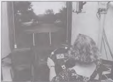
The VIDSIM is equipped with three widescreen projection TVs. A monitor (to the right) gives directions on screen.
