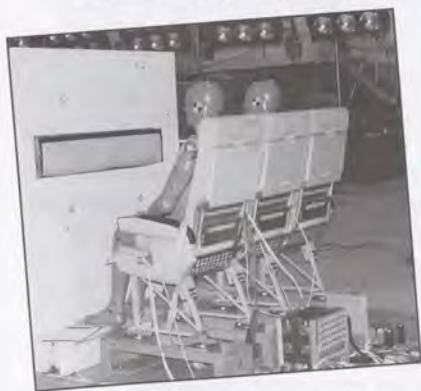
The photo shows the setup for an airplane seat test, commonly referred to as a sled test.
