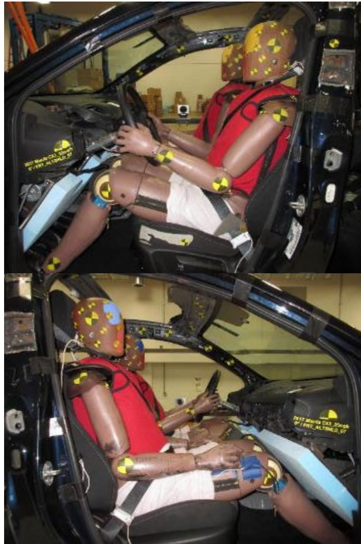
Figure 46. THOR-50M Driver (top) and passenger (bottom) seated for test
