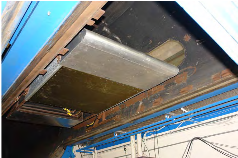
Figure 5.3 Wing tank in the high speed test section of the wind tunnel
