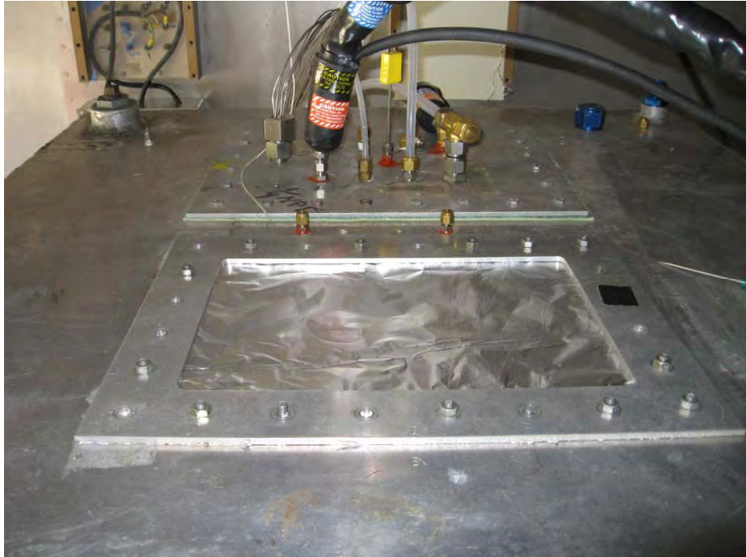
Figure 3.2 Fuel tank instrumented with thermocouples and hydrocarbon analyzer sample lines
