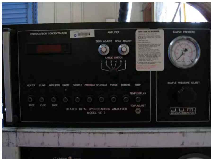
Figure 3.3 Flame ionization detector hydrocarbon analyzer
