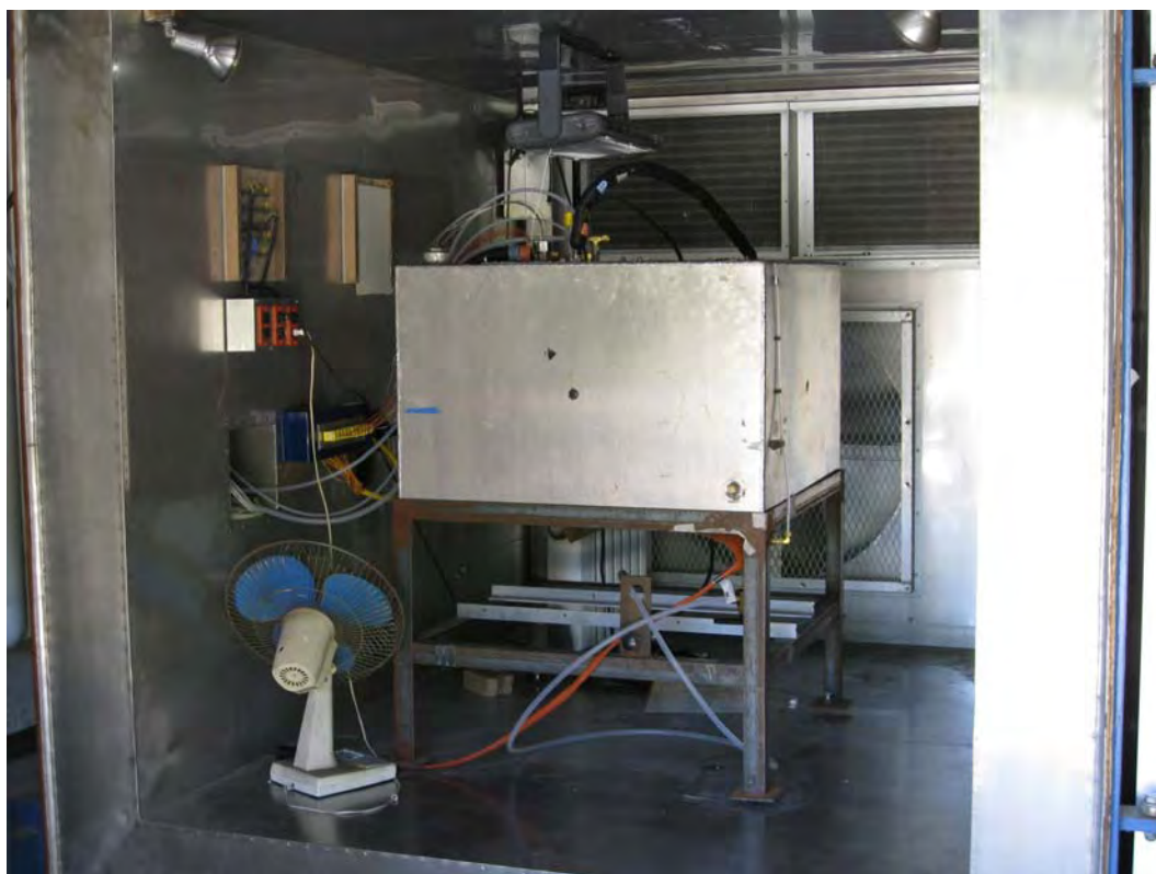
Figure 3.1 Fuel tank placed in the altitude chamber
