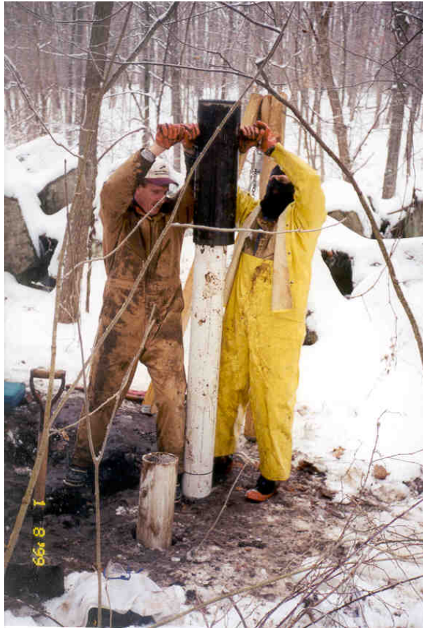
Figure 2. Soil sampling for site characterization for phytoremediation site clean-up in Bedford, Indiana.
