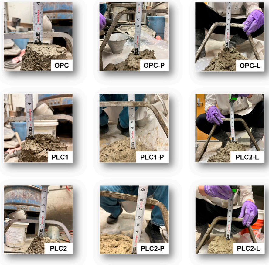
Figure 3.4 Photos of the Slump Test.
