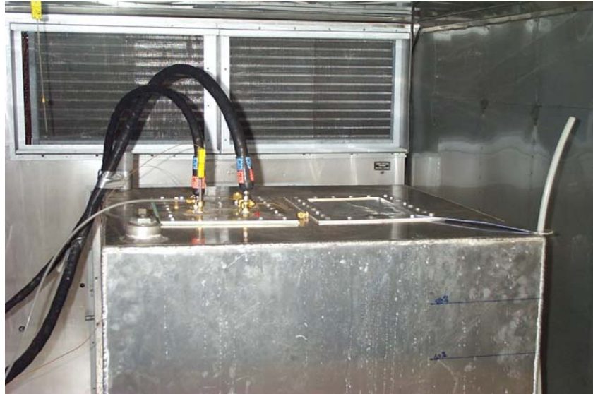
Figure 3.1. View of top surface of fuel tank. Heated sample lines are the black hoses connected to the sample panel.
