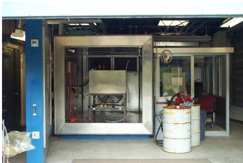
Figure 3.2. View of the fuel tank inside the environmental chamber. The fuel drums used for fill and drain are in the foreground. The control booth is to the right of the chamber.
