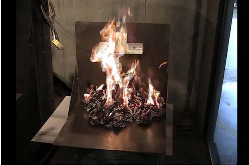
Figure 4. Fire at the Outset of Each Paper Towel Burn Test
