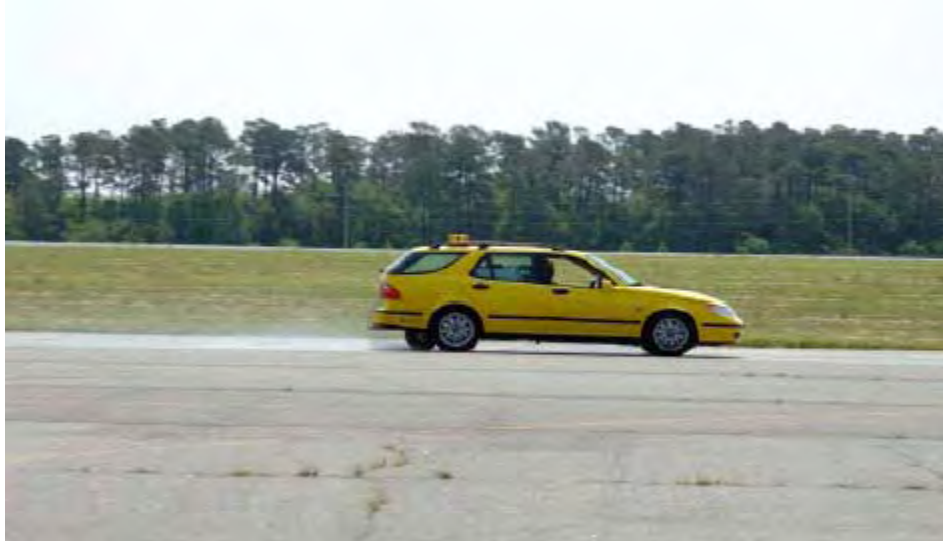
Figure 18. Saab Sarsys Friction Tester in Action
