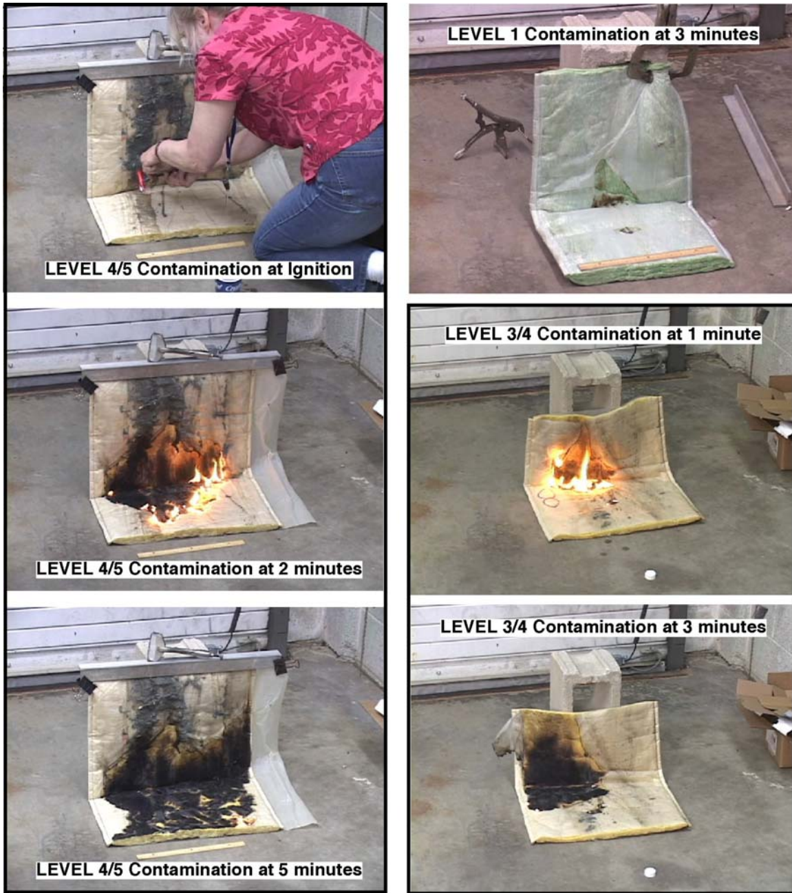
Figure 9. Flame Spread Test Results at Different Ignition, Midway Through the Test, and at Flame Extinction for the 2702 Sample (L = 4/5), the 4606 Sample (L = 3/4), and the 2383 Sample (L = 1)
