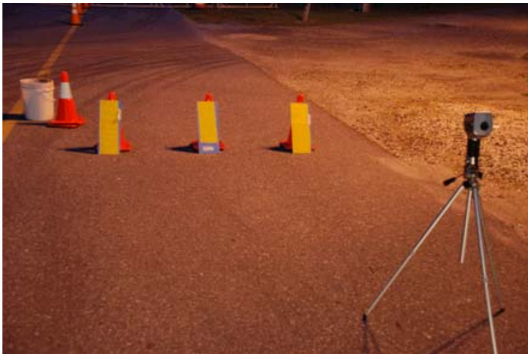
Figure A-6. Luminance Measurements of Retro-Reflective Panel Setup
