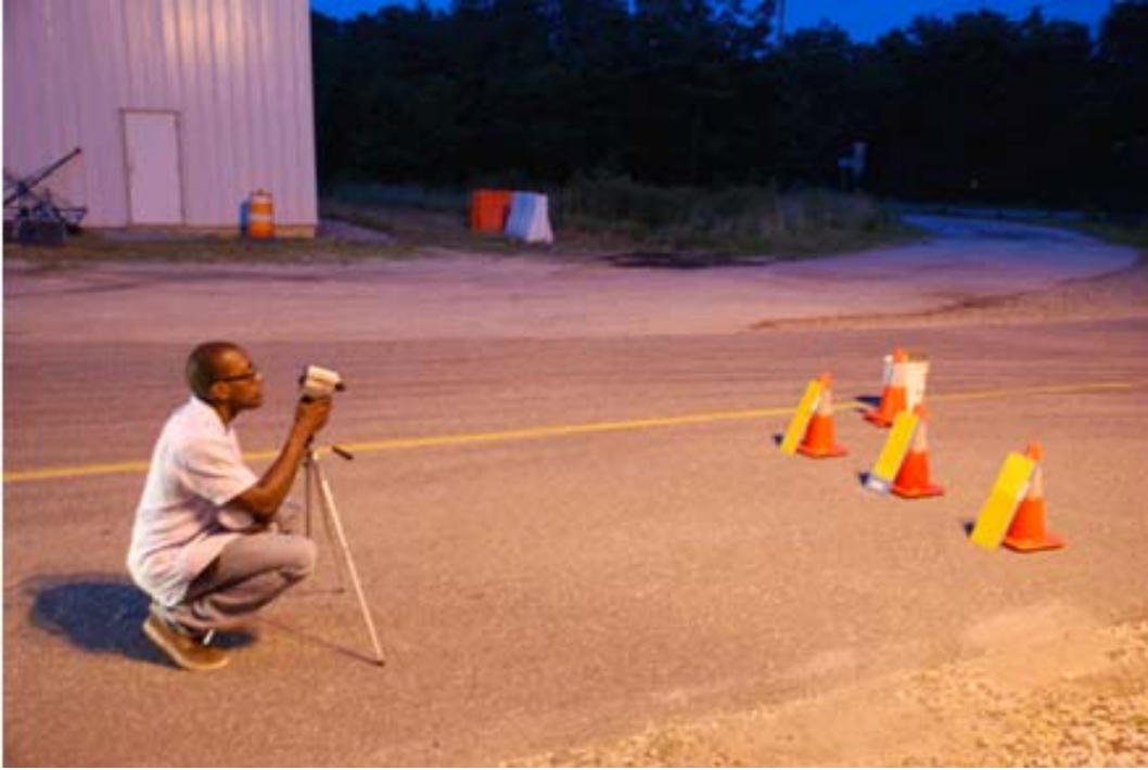
Figure A-7. Luminance Measurements of Retro-Reflective Panels
