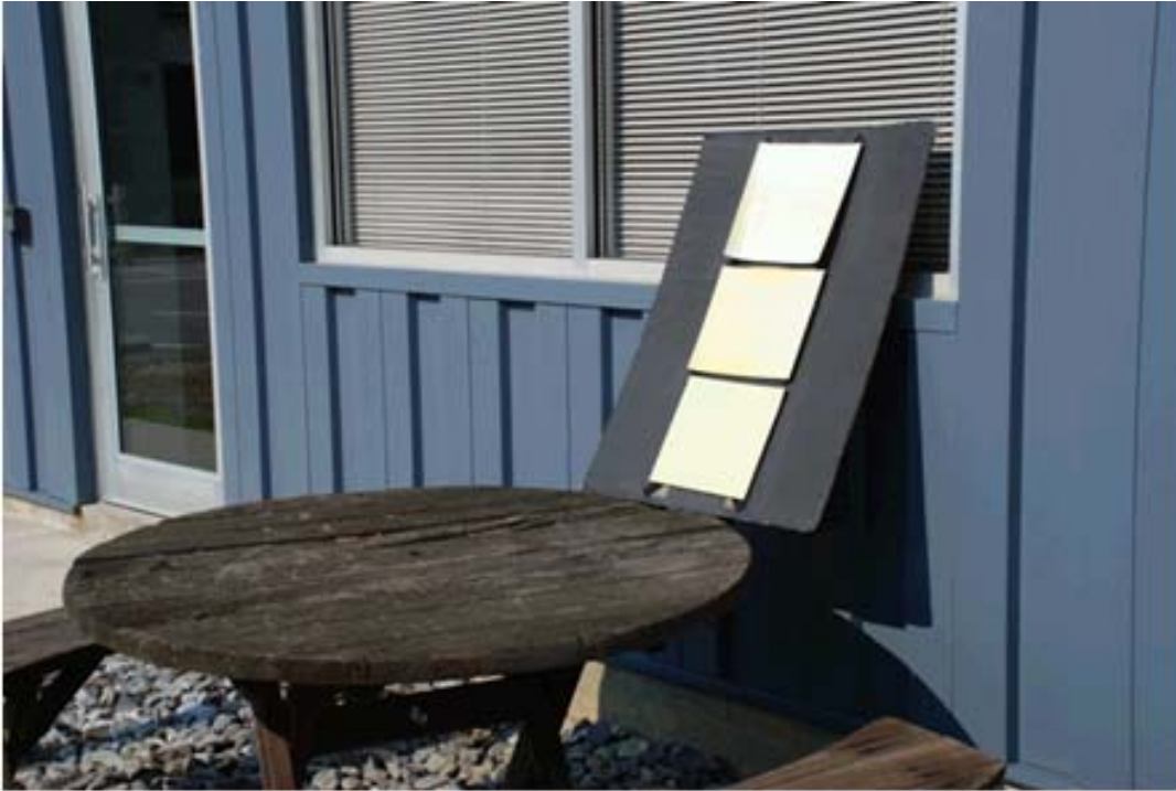
Figure A-1. Test Panels Charging Under Sunlight
