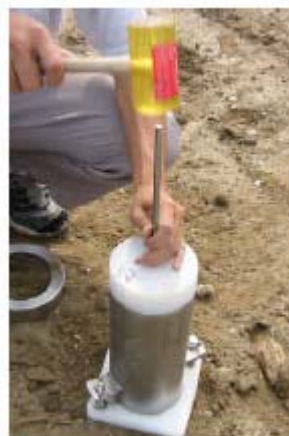
Fig. 5.9 Driving the Center Rod through the Rod Guide
