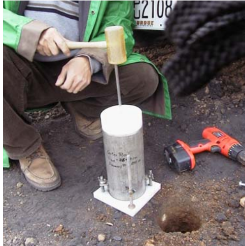
Fig. 3.7 Photo of Guide for Installing Center Rod
