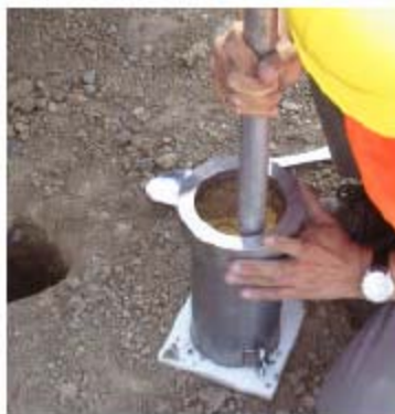
Fig. 5.7 Place MRP Head on Mold Using Adapter Ring
