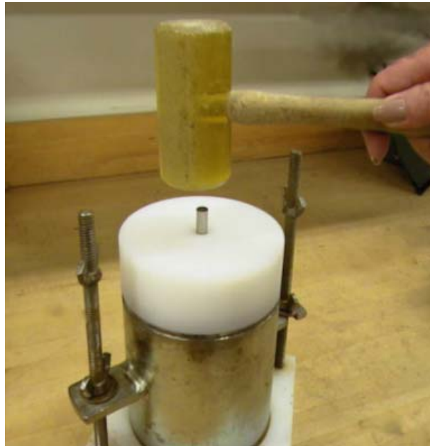
Fig. 8.1 Driving the Central Rod through the Rod Guide Placed on Mold
