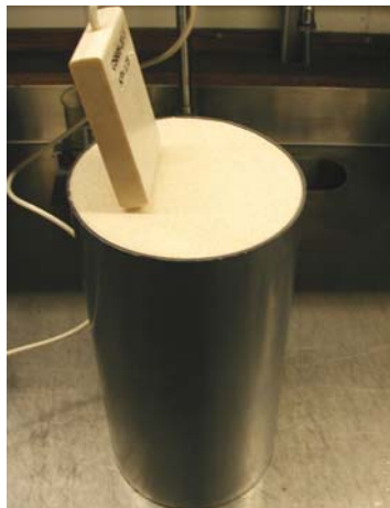
Fig. A2.6. Fully Embedded CSI 605 Probe
