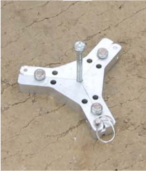
Fig. 8.4 Field Test Procedures: (a) Spikes Being Driven through Template into Soil Surface; (b) Multiple Rod Probe Head on Spikes for TDR Measurement
