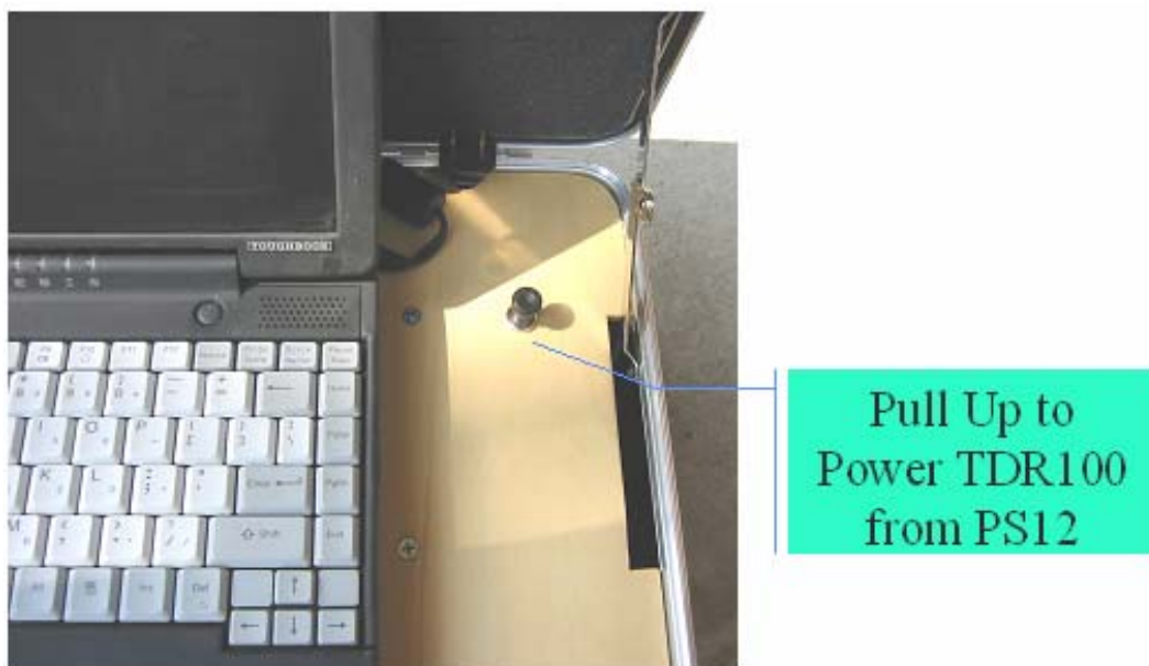
Fig. 3.18 Pull Switch to Supply Power to TDR100 from PS12 Power Supply
