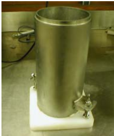
Fig. 3.8 Photo of Compaction Mold with Height Twice That of the Standard Compaction Mold
