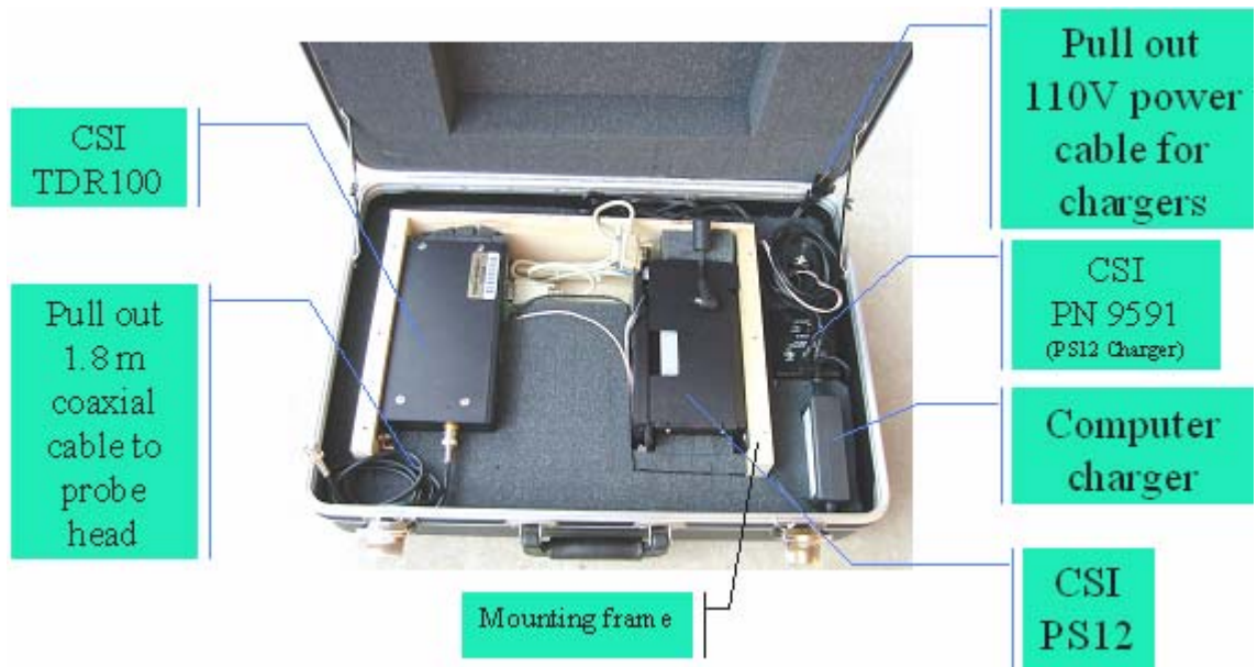
Fig. 3.17 Layout of TDR100 and Power Sources in Case
