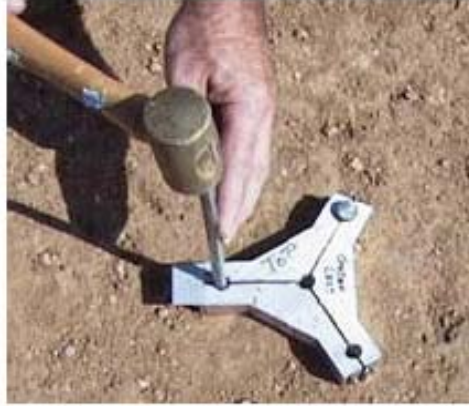
Fig. 5.1 Driving Probes through Template for the Field Test
