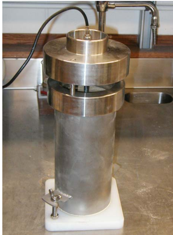
Fig. A2.10 TDR Test in a 4.0-in Diameter by 9-in. High Metal Compaction Mold
