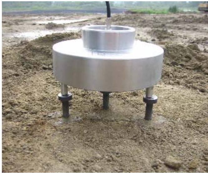
Fig. 6.8 Field Test Procedures: (a) Spikes Being Driven through Template into Soil Surface; (b) Multiple Rod Probe Head on Spikes for Measurement
