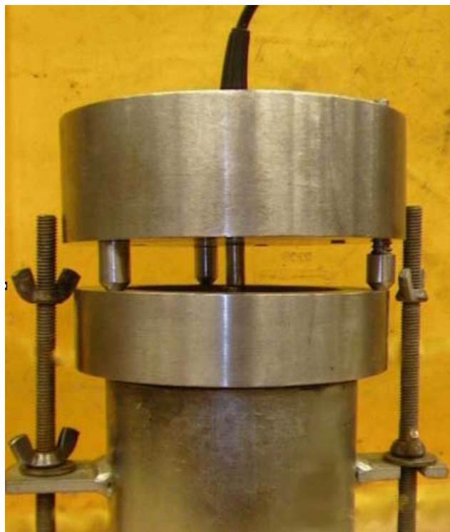
Fig. 6.6. Mold test procedures (a) Driving Central Rod through a guide placed on the mold (b) Multiple Rod Probe Head ready for making TDR measurements
