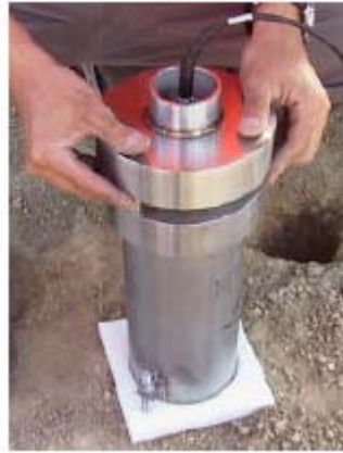
Fig. 5.10 Placement of the MRP Head on the Adapter Ring
