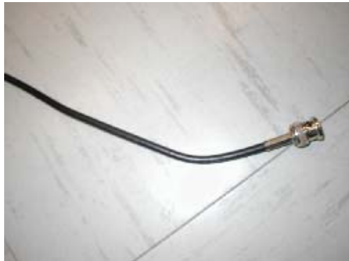
Fig. 3.4 Coaxial Cable with Impedance of 50 ohms
