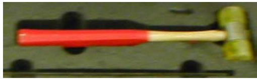
Fig. 3.12 Hammers: (a) Insitu Probe Rod Installation; (b) Mold Rod Installation
