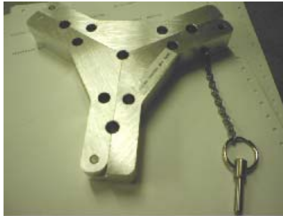
Fig. 3.6 Photo of Guide Template for the Multiple Rod Field Probes
