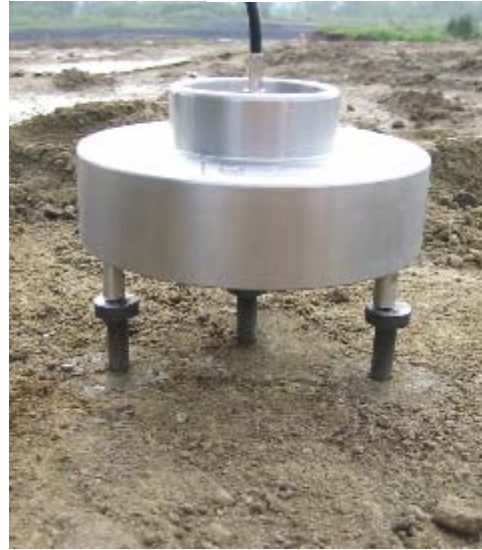
Fig. 8.4 Field Test Procedures: (a) Spikes Being Driven through Template into Soil Surface; (b) Multiple Rod Probe Head on Spikes for TDR Measurement
