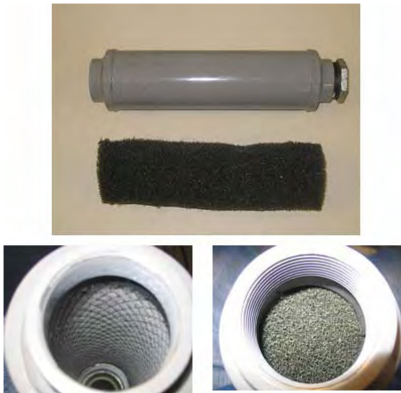
Figure 7. The Muffler Section Without and With a Foam Insert
