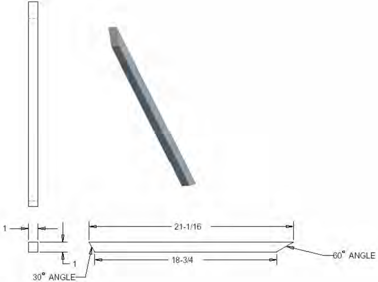
Figure A-22. Dimensions of the Support Members (All dimensions are inches.)
