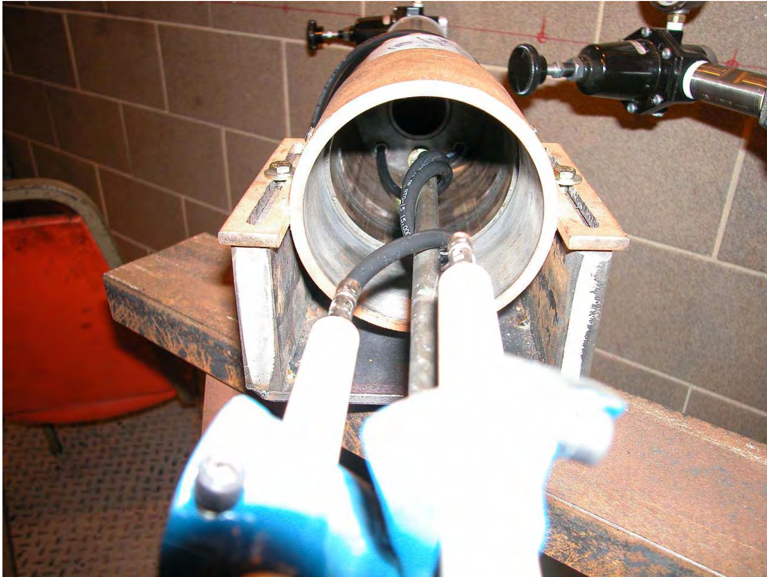
Figure A-8. Photograph of the Igniter Wires From Above
