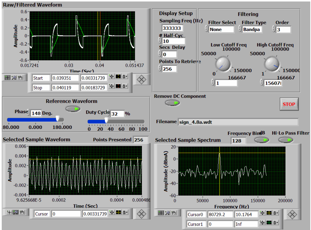
Figure A-13. Spectrum at 4.8 amps Just Before Conduction
