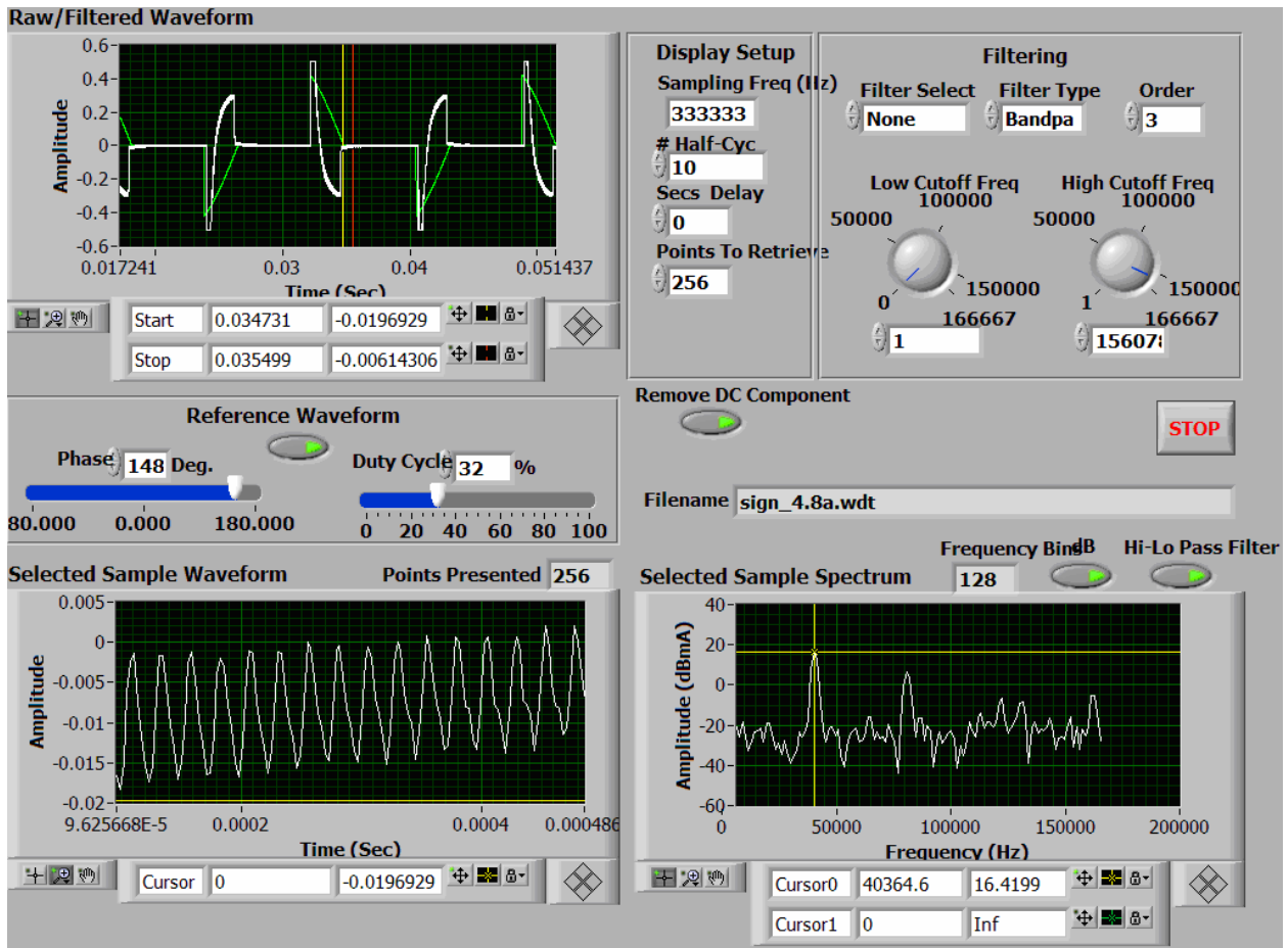
Figure A-12. Spectrum at 4.8 amps Just After Conduction
