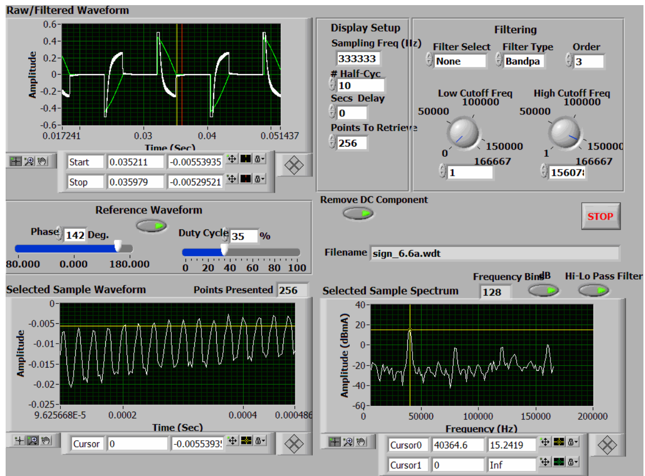
Figure A-3. Spectrum at 6.6 amps Just After Conduction
