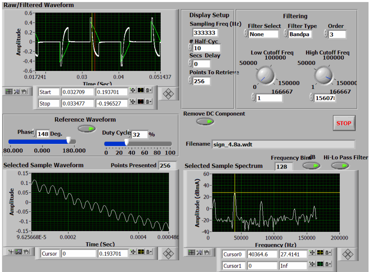
Figure A-11. Spectrum at 4.8 amps During Conduction
