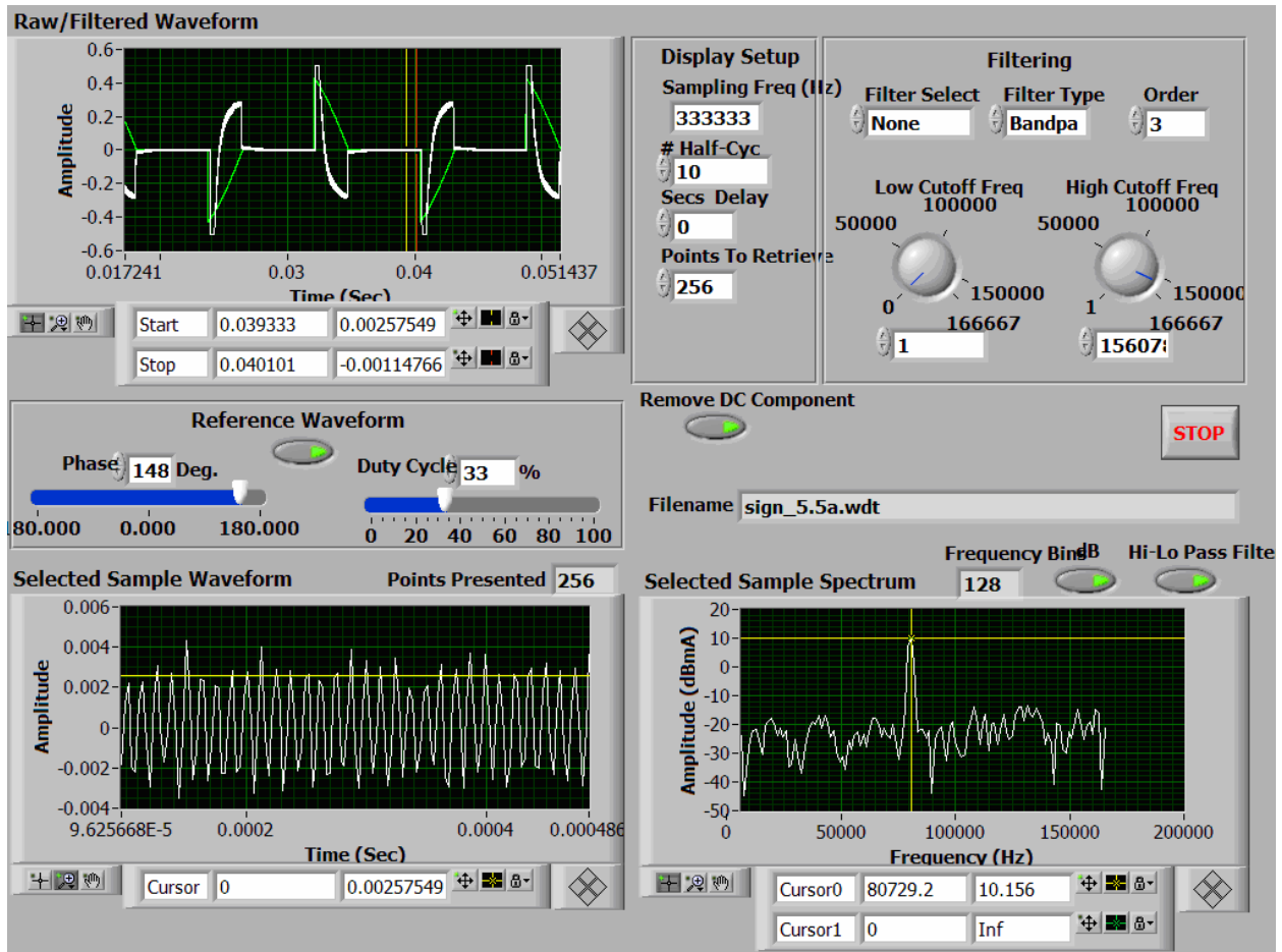
Figure A-7. Spectrum at 5.5 amps Just Before Conduction
