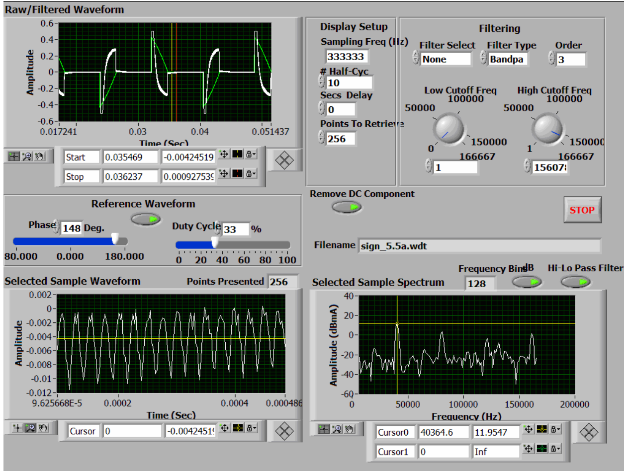
Figure A-6. Spectrum at 5.5 amps Just After Conduction
