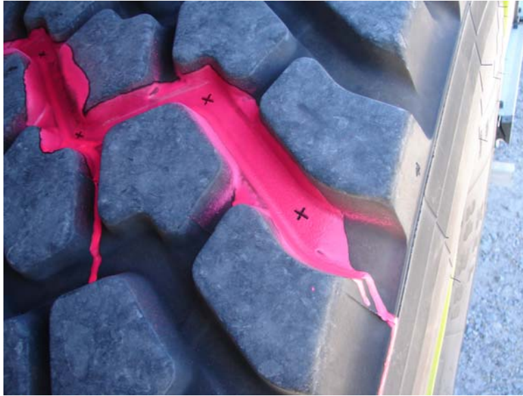
Figure 4. Paint Markings Used to Identify Tread Measurement Points
