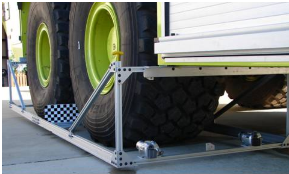
Figure 2. Rear Wheels on FAA 6x6 Research Vehicle Showing Cameras and Measurement Reference Locations
