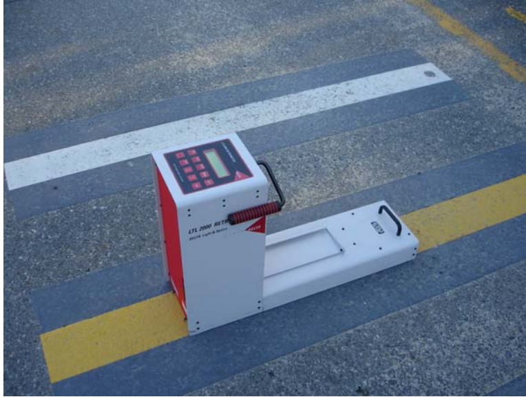
Figure 18. Retro-Reflectometer, 30-Meter Geometry for Measuring Retro-Reflectivity of the Glass Beads
