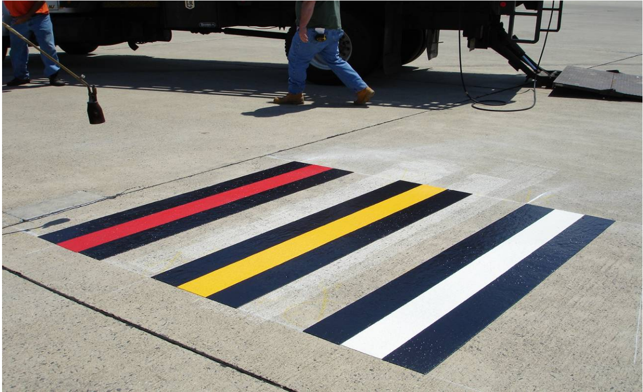
Figure 2. Red, Yellow, and White Stripes on PCC at FAA William J. Hughes Technical Center
