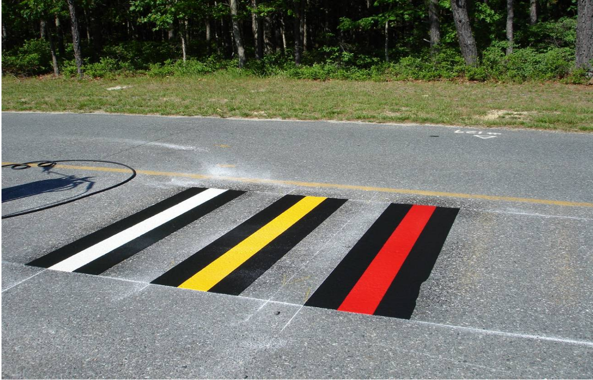
Figure 6. White, Yellow, and Red Stripe on HMA at FAA William J. Hughes Technical Center
