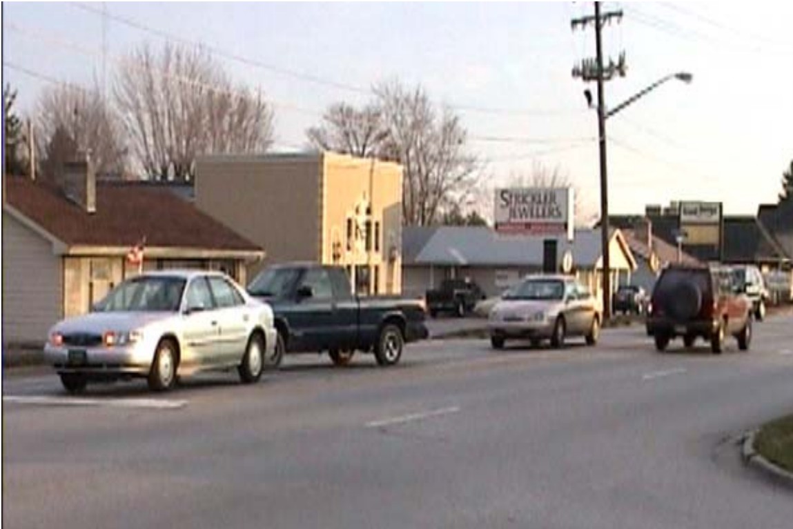
Figure 8.1 Frequent lane changing due to blocking of lanes by left turning vehicles
