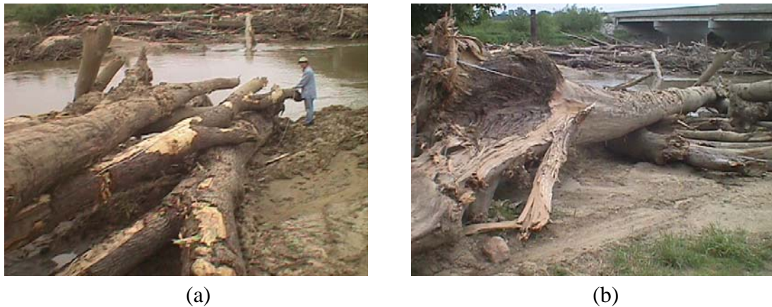
Figure 5.9: Logs taken from debris pile: a) 42-ft log being measured, b) longest log (length, 67.7 ft) measured
