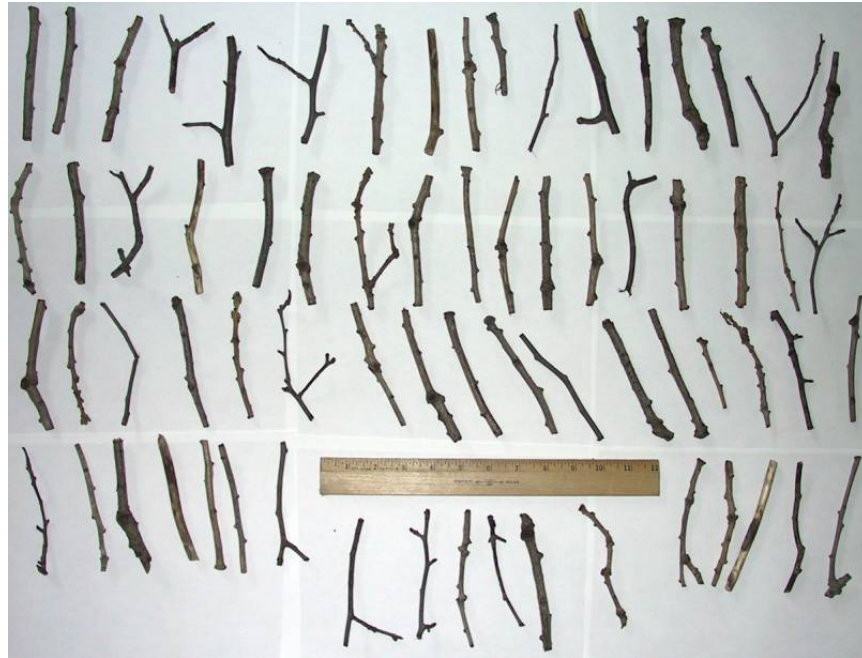
Figure 2.1: Twigs used as model logs
