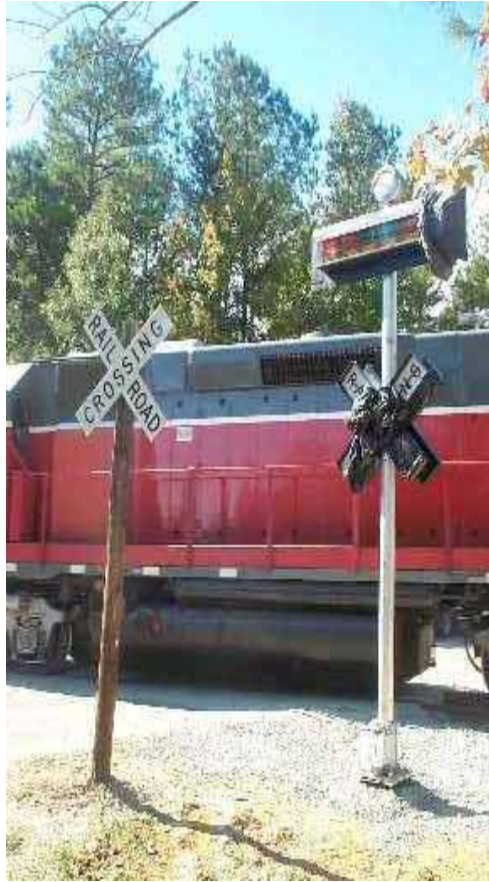
Figure 6. EVA Signal System Corporation Warning Device Configuration as Tested in North Carolina (Jennings, Field, Worley, and Scott, 2005)
