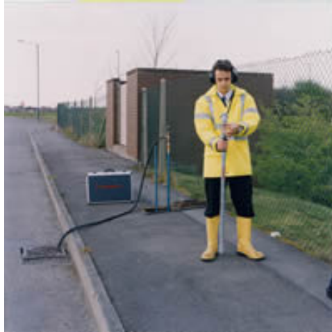
Figure 7.22. Application of Acoustic Pipe Tracer (RD 500)
