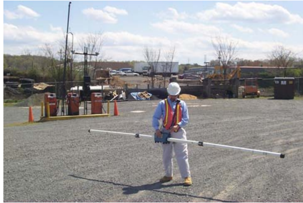
Figure 5.16. Application of Terrain Conductivity Method (Source: So-Deep Inc)
