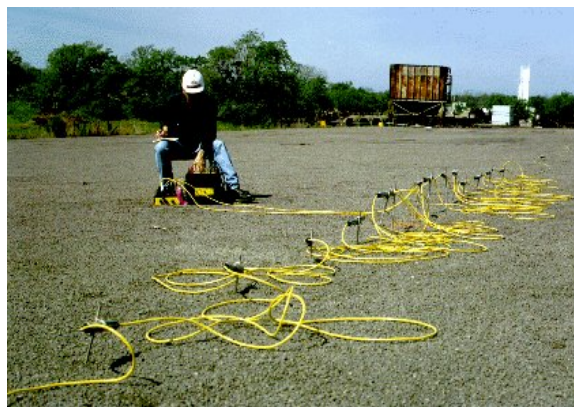
Figure 5.26. Application of resistivity method (Source: http://www.geop.ubc.ca )
