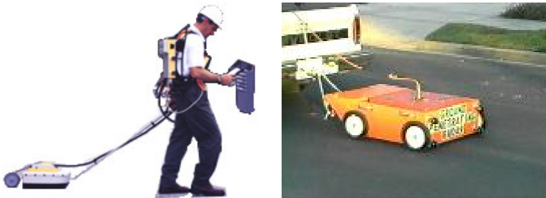
Figure 5.18. GPR Application by Hand and by Truck
