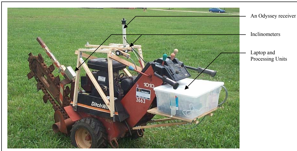
Figure E3.4. A trencher and SPS-CAD
