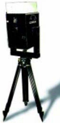
Figure 3.6. The CYRAX Laser-Mapping and Imaging System (Wilson et al. 1998)
