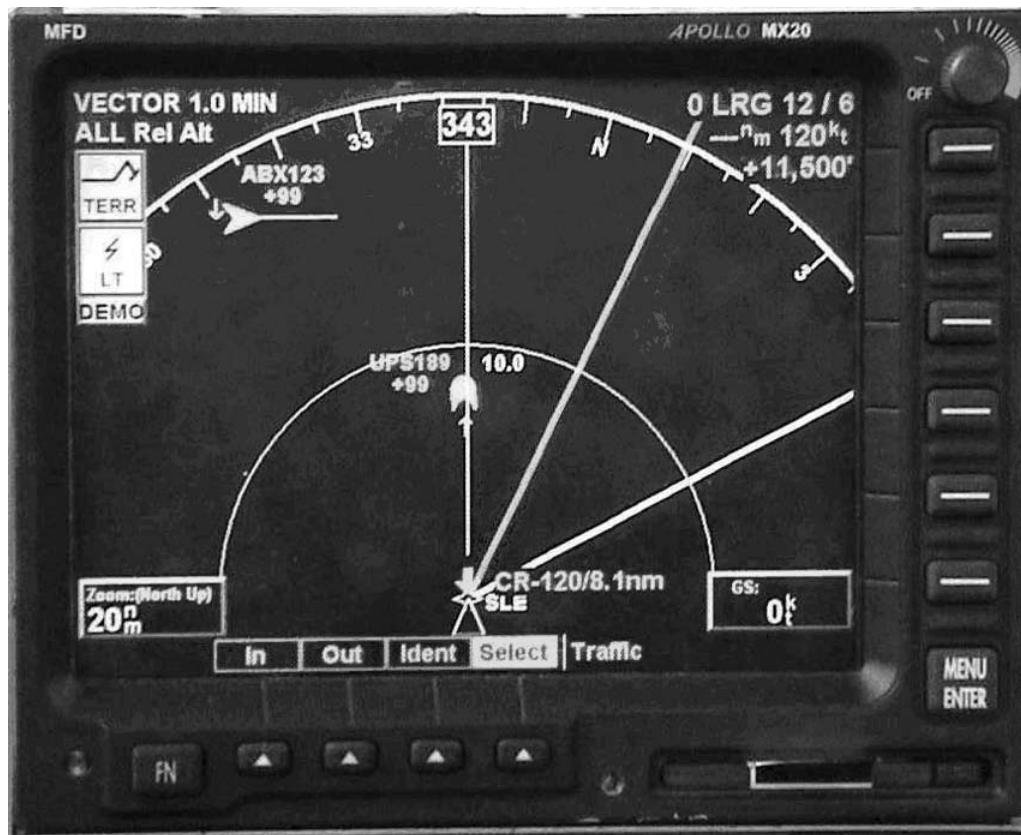
Figure 1. Range Monitor: Garmin International's MX-20™ user interface enhanced.
