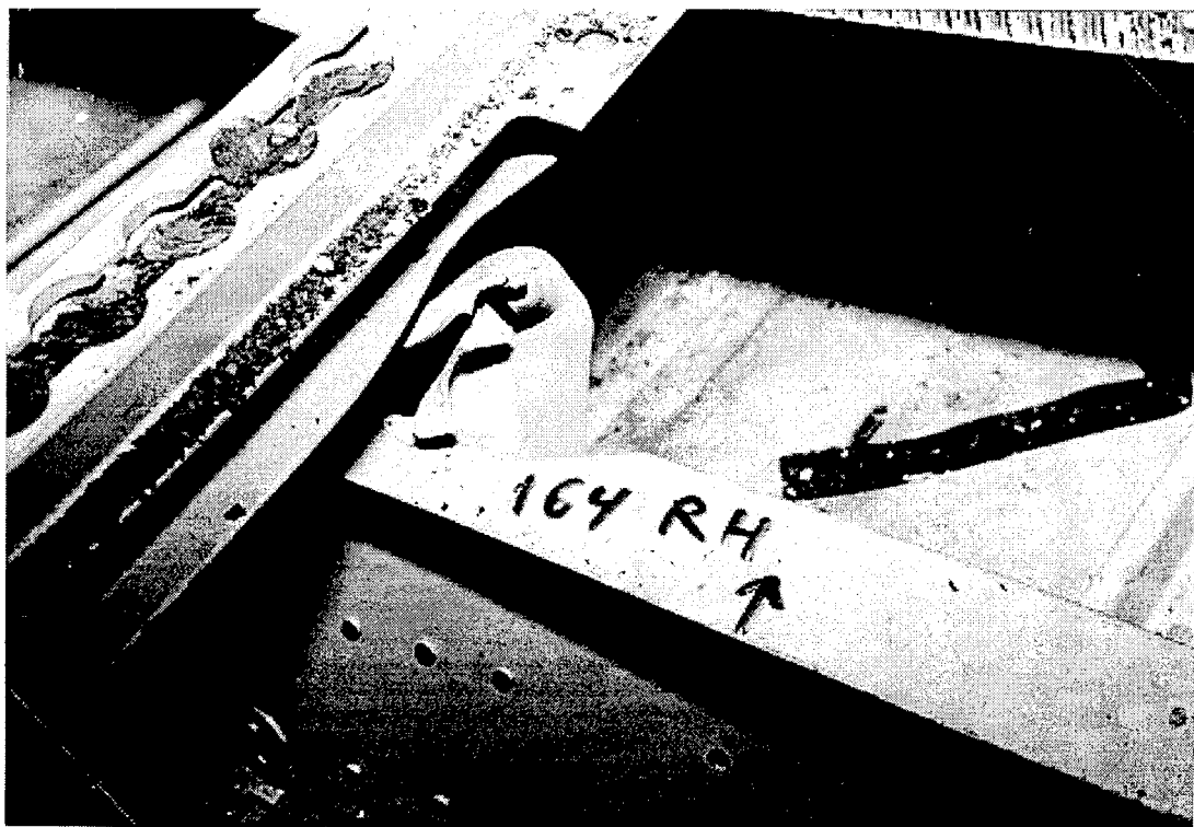
FIGURE 6. UNDERFLOOR BUCKLING RIGHT-HAND SIDE AFTER IMPACT
