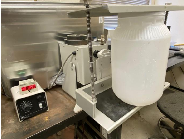
Figure 5.3: Glas-Col's Dry Powder Rotator for the Idaho Degradation Test
