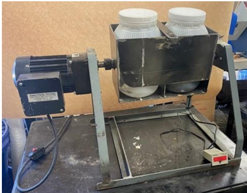
Figure 5.4: The Idaho Degradation Testing Apparatus
