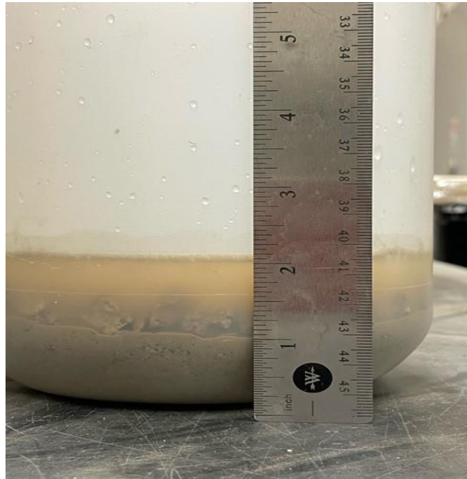
Figure 5.6: Water Amount (350 g) to achieve \frac{1}{2} in. coverage
