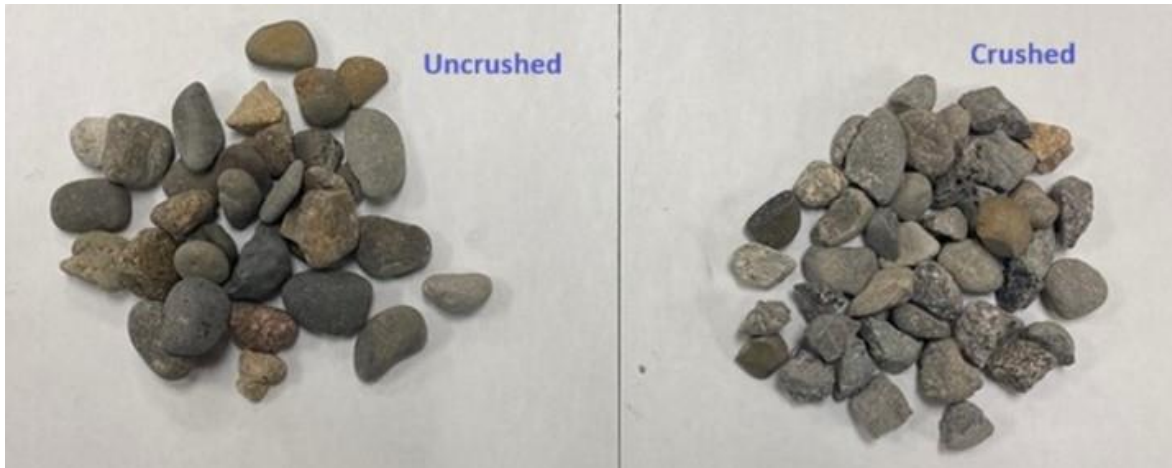
Figure 6.16: Crushed and Uncrushed Aggregates (Fr-76s)
