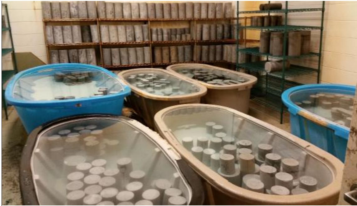
Figure 2.32 Saturated Lime-water baths for Curing at Room Temperature (73°F) (Georgia DOT 2016).
