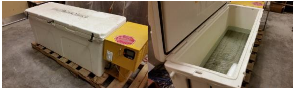
Figure 2.33 Intellicure Temperature Controlled Curing Box for High Temperature (140°F) Curing (Georgia DOT 2016).
