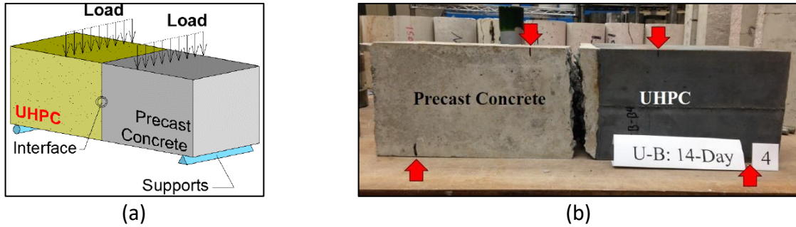
Figure 2.22 (a) Flexural test based on ASTM C78, (b) photo after failure (FHWA 2018).
