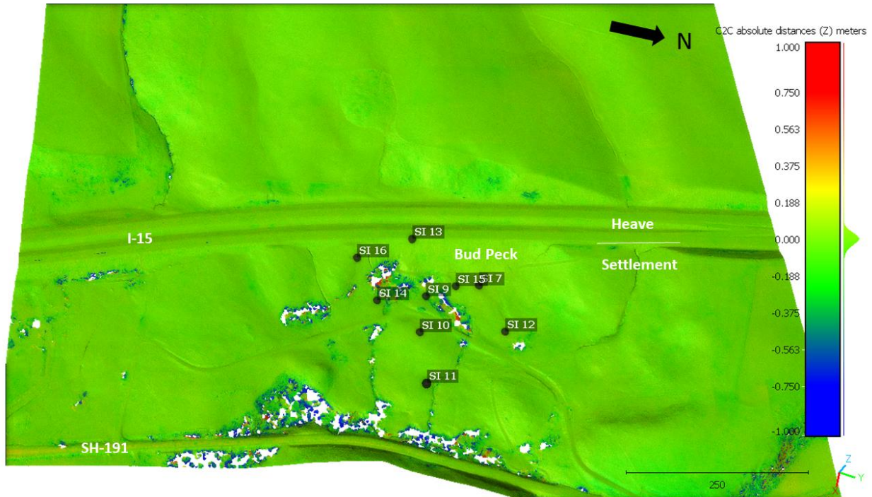
Figure 3.47 Ground Surface Displacements Between the ISU September 2023 and October 2024 UAS Surveys
