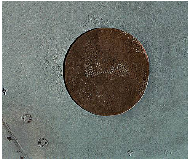
Figure 13. Composite-Bonded Patch Failure Showing Interfacial Failure Between Adhesive and Patch Surface due to Presence of a Silicone Release Agent on Peel Ply 2
